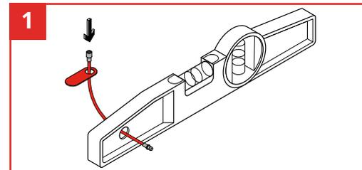
Feed the Gripplock Cable through the pre-formed hole in the tool.
