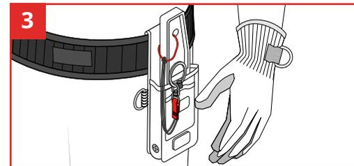
Your Gripplock Cable is now ready to be connected with a suitable GRIPPS® tether.
