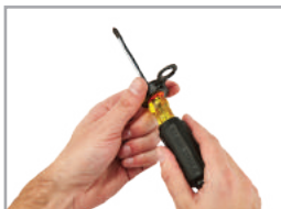
SLIDE THE SLIP INTO PLACE
