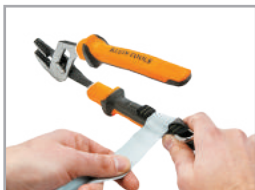
WRAP TAPE AROUND TOOL & TAIL
